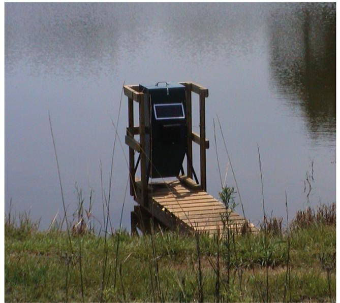
Figure 8. A fish feeder, placed on a dock for easy access, is activated by a timer and solar powered.
